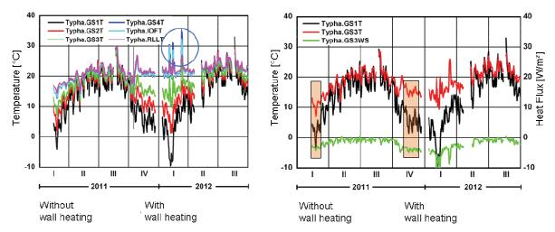
Fig. 5. Measured course of the temperature as daily mean values for the period from January 2011 to September 2012 (left) and heat flow measured behind the internal insulation (layer 3) with course of the temperature at layer 1 and 3. The bars show time periods suited for assessing the thermal resistance (right).
