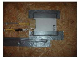
Fig. 4. Outer sensors at layer 1 beneath the outside rendering (left) as well as Temperature sensor, heat flow wafer and humidity sensor on barrier layer 3, beneath internal insulation on the second insulation board layer (right).
