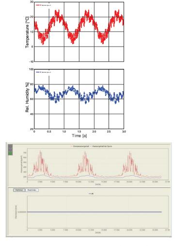
Fig. 8. Course of temperature (top) and relative humidity (bottom) between external wall and internal insulation at a back flow of 1  $m^3/md$  (left) and calculated results by WUFI®-Bio for the area behind the internal insulation.
