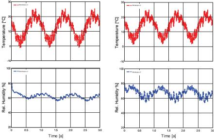
Fig. 7. Course of temperature (top) and relative humidity (bottom) between external wall and internal insulation with careful implementation (left) and without perfect tightness with back flow of 1 l/mh (right).
